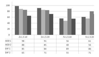
Fig. 4.The effect of liquid-to-solid ratio on Zn and Fe yield -%, 1.5 M, 30°C, 120 min
