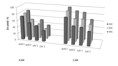
Fig. 2. The effect of temperature and acid concentration (in mol/dm<sup>3</sup>) on Zn dissolution (L:S=10, 120 min)
